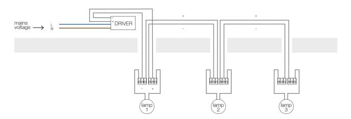
the cable between the lamps is not supplied, it is recommended to use one with a minimum section of conductors of 1 mmq
